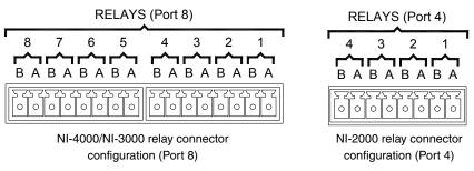
FIG. 14 RELAY connector (male) (NI-4000/3000/2000)
